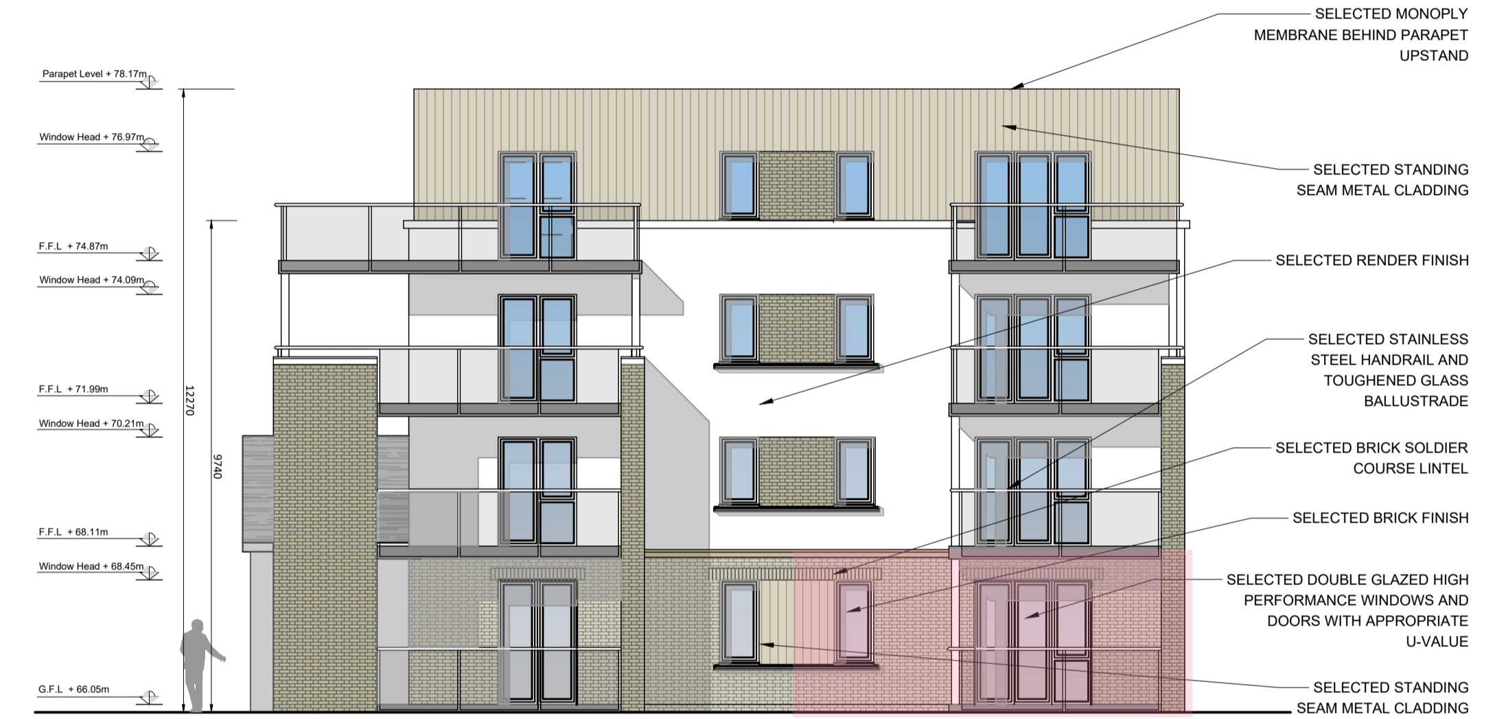
Block C - North-east Elevation
