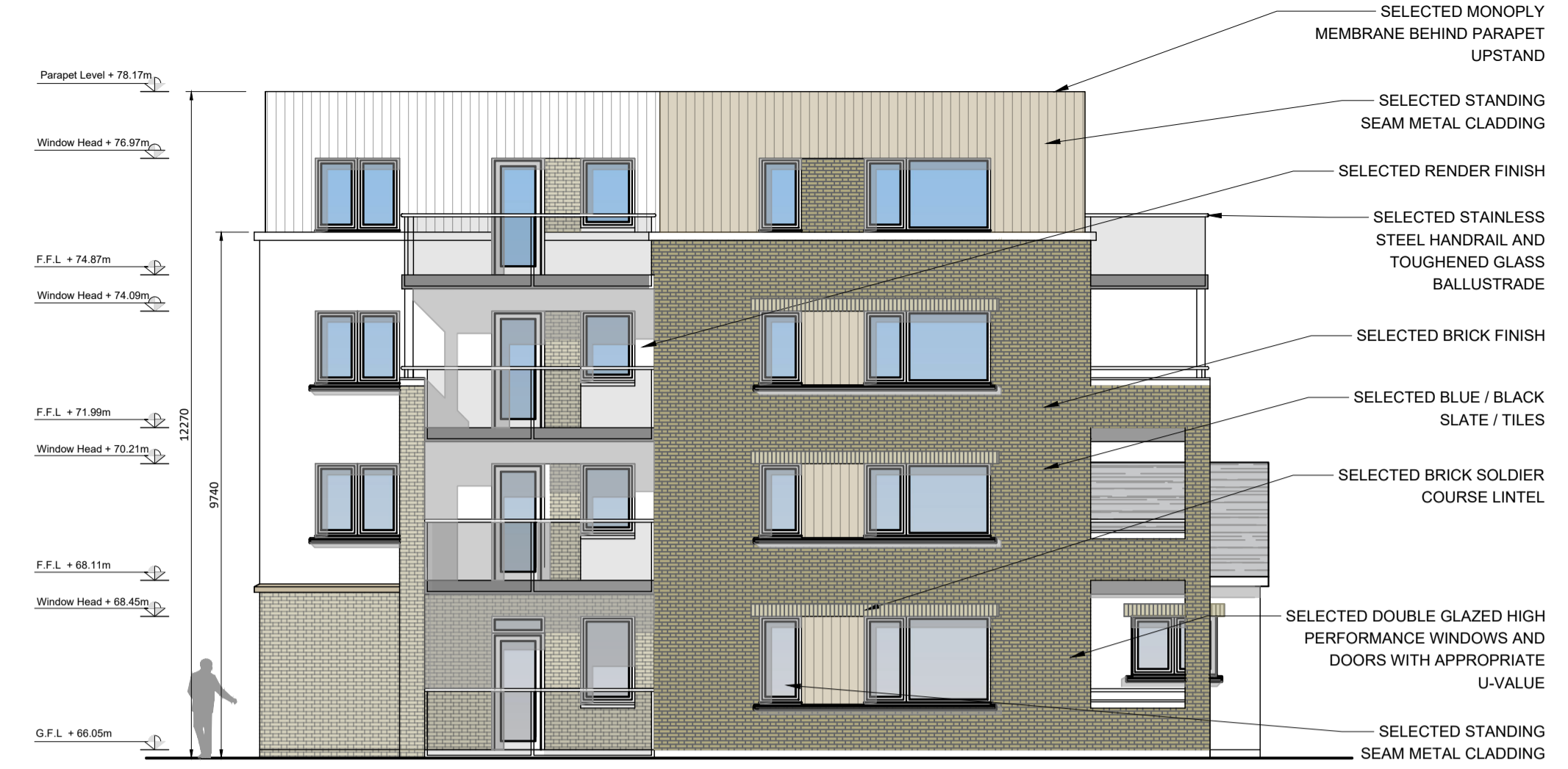
Block C - South-west Elevation
